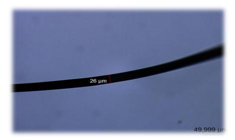
Microscopic image of a filament removed from the original PET textile waste.
