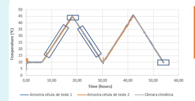
Test Cell 1 - Sample with PCMs Test cell 2 - Sample without PCMs Climatic chamber - Ambient temperature
