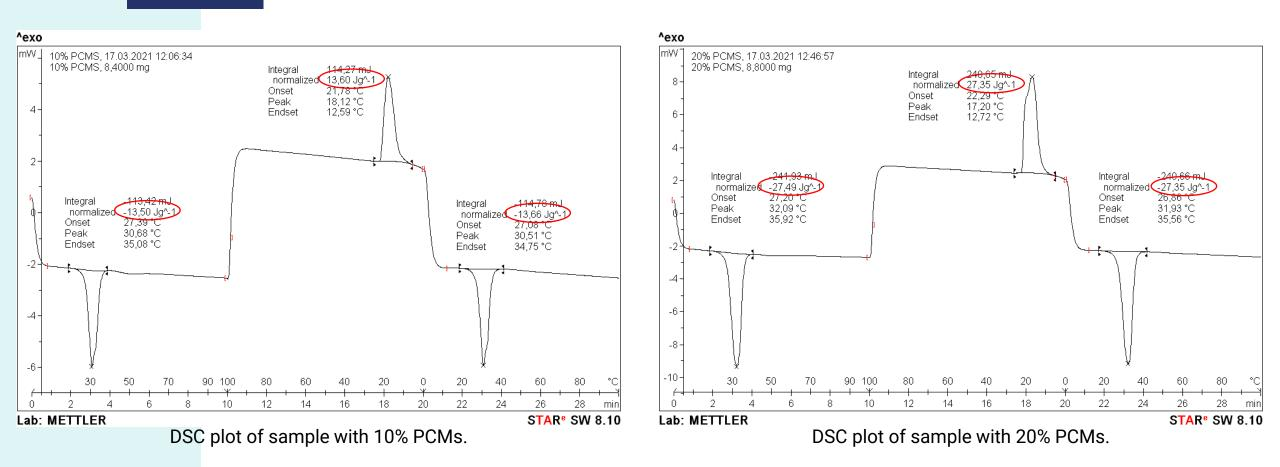
With the increasing percentage of PCMs from 10% to 20%, the latent heat of fusion and crystallization doubled.
