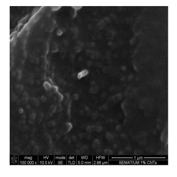
Cross section of the PET40\_rPET60\_1CNT's sample.
