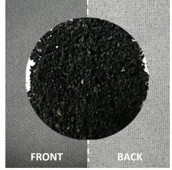
Application of high temperatures, above the  $T_m$  of the materials, to put the residues in a molten state, allowing their agglomeration. After agglomeration, the residues are cooled, becoming rigid.
